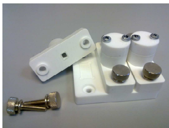
Figure 6.7. Fabricated immobilization cells for LW devices.
