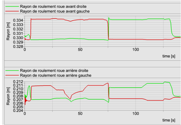
Figure 9: Original tramway on straight track: flange + tread contact
