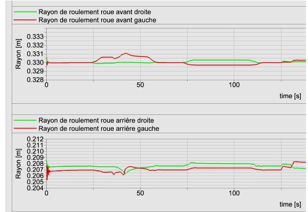
Figure 9: Original tramway on straight track: flange + tread contact
