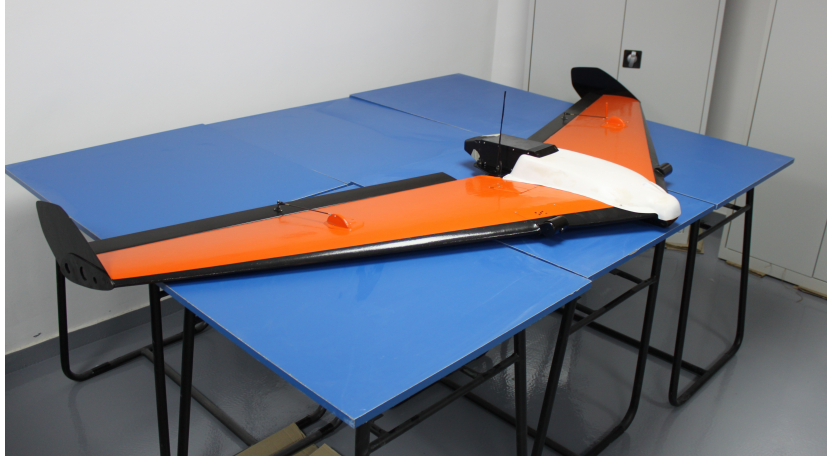
Figure 8.7: The Unmanned Aerial Vehicle built by Reeve River Aerospace and dedicated to the SWING payload. It is electrically-propelled and can reach 3 km altitude with its 2.5 m wingspan. The typical speed is 60 km/h.
