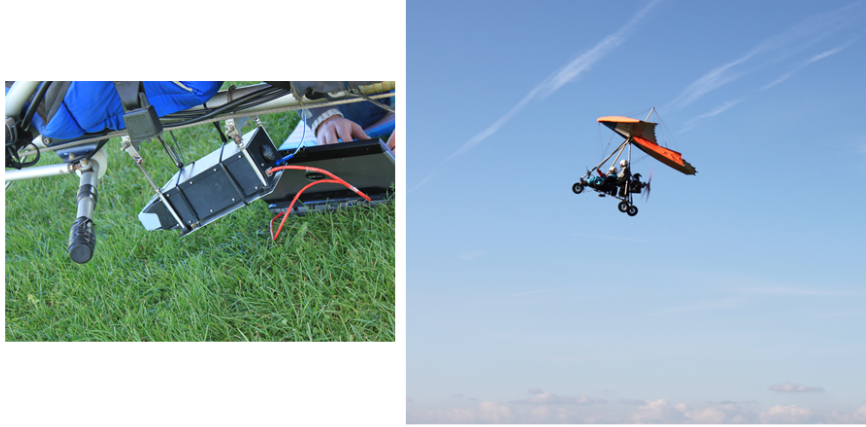
Figure 8.8: Installation of SWING on an ultralight and illustration of the test flight on 28 October 2012.
