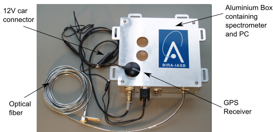
Figure 6.2: The ULM-DOAS instrument. Inside the box are a compact UV-Vis spectrometer and a PC-104. Light is collected directly by the optical fiber and a GPS is used to geolocalize the measurements. The whole system is powered with 12\text{ V} .
