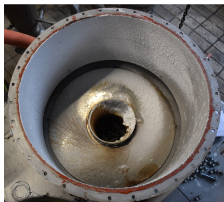
(a) Bottom part of the spray drying chamber with the central hot air inlet
