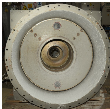
(b) Top part of the spray drying chamber with centrally the passage to the cyclonic extension and all the way at the top the main air outlet
