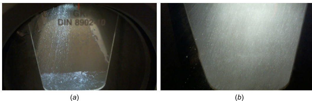
Fig. 3 The droplet size and distribution was monitored visually through the saturation tower loop holes. The injected water flow rate and droplet distribution from (a) corresponds to the low flow rates and low injection pressure, while (b) shows the water flow rate and distribution after increasing the injection pressure.
