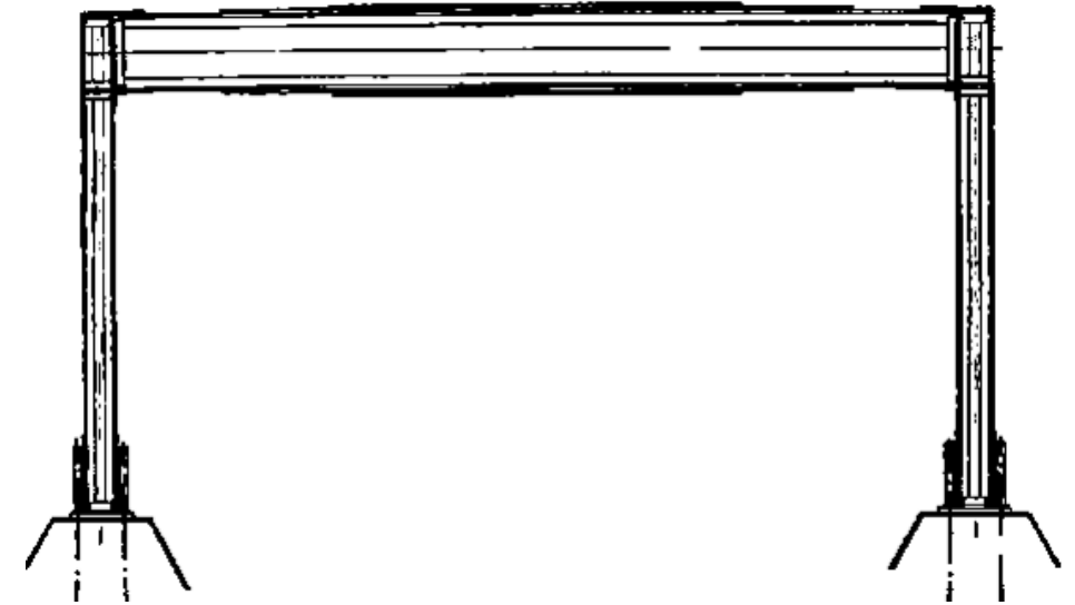
a portal frame fixed at both ends
