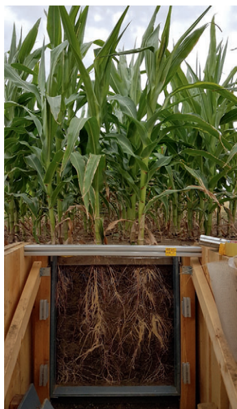
Figure 6: Root windows allowing visual monitoring, as well as repeated and non-destructive access to field-grown maize roots during the entire vegetation period. Idea and design: Eva Oburger, BOKU—University of Natural Resources and Life Sciences; Technical construction: Gottfried Wieshammer (gottfried.wieshammer@aon.at), Technisches Büro für Bodenkultur, Austria.
