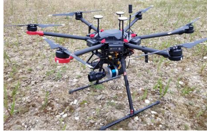
Figure 1. DJI Matrice 600 carrying the YellowScan Surveyor LiDAR sensors that was used in this study
