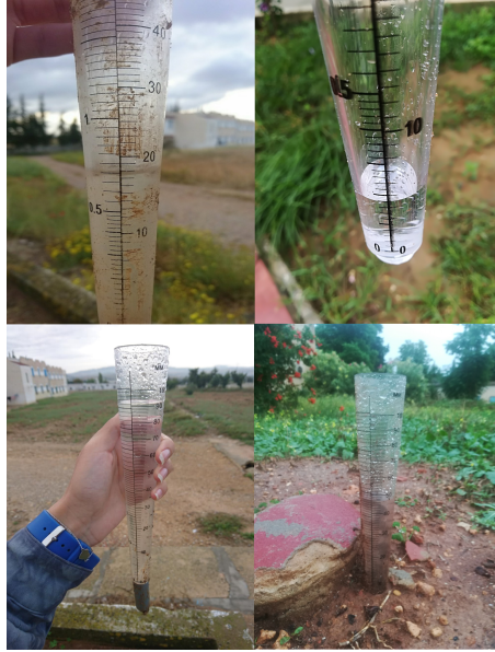
Figure 4.9: Photos of rain gauges sent by citizens during monitoring rainfall in the test region.
