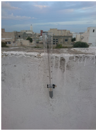
Figure 4.3: Rain gauge fixed by a citizen scientist during monitoring rainfall.
