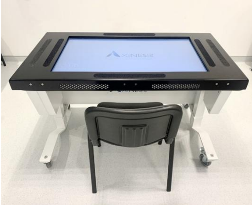
Figure 1. The non-immersive VR device. The REAtouch® system consists of a 43-inch interactive touchscreen mounted on an adjustable support structure allowing customization of height and inclination. In the present study, the screen was positioned horizontally ( 0^\circ inclination). Participants interacted directly with the touchscreen to perform the visual search task. Photograph taken by the authors.
