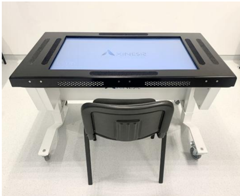
Figure 1. The non-immersiveVR device. REAtouch® (Axinesis®) touch-sensitive 43" screen tablet with multisensory and real-time performance feedback. The height and inclination of the screen can be adjusted. In the present study, the inclination was the same as that presented here (i.e., 0°).
